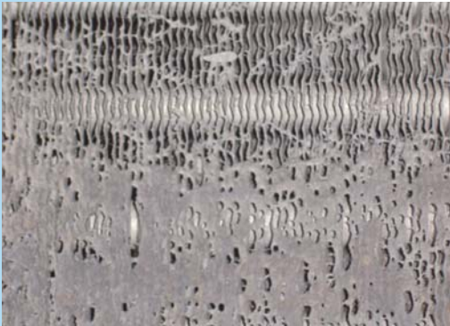
Coil before AerisGuard treatment
