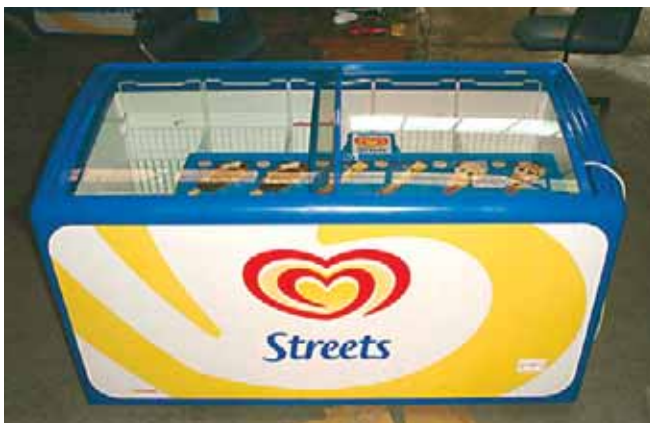
A hydrocarbon ice cream freezer from the Unilever field test at the Sydney Olympics
