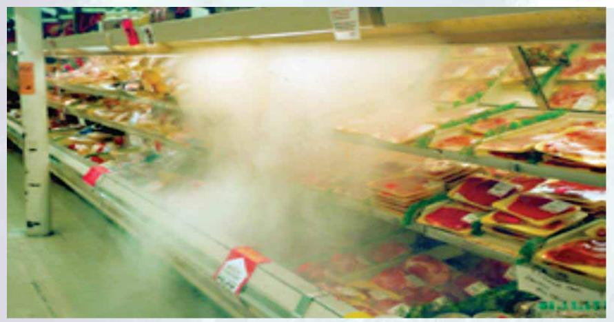
Smoke curtain demonstrates cold air spilling from supermarket open display case
